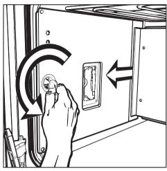
■ Unscrew the fixing using a coin.
